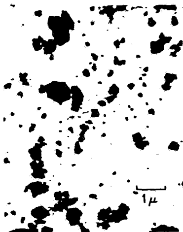
Figure 2. Dust removed from brake drum.
