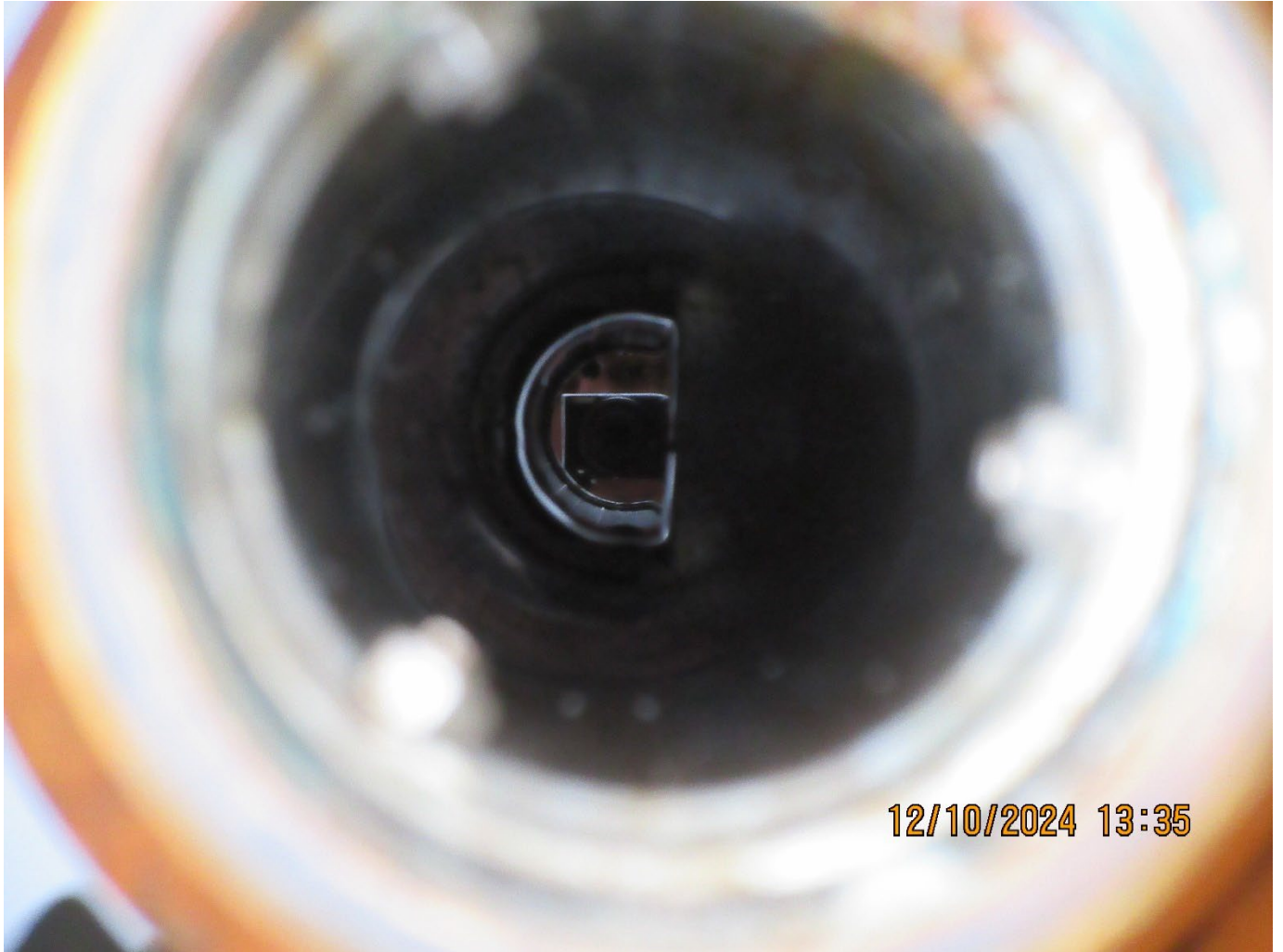
Photo 13 – Fuel port interior with flapper valve as seen from above.
