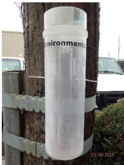
Photo #:01 Description: Facing east, photo of rainfall gauge located on-site.
