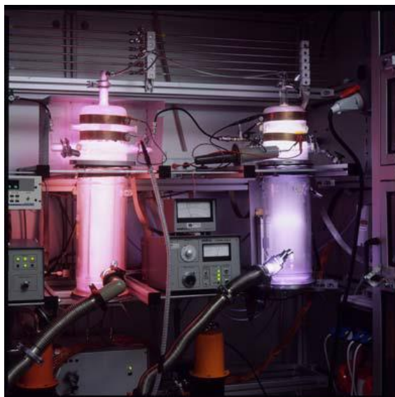
Figure 5: Two of RISE small plasma reactors, upper electrode
