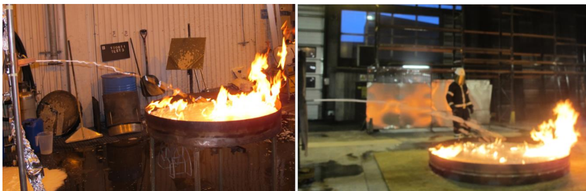
Figure 13. SP Method 2580 (left) is a down-scale of the larger test according to the European standard EN 1568-3 (right).
