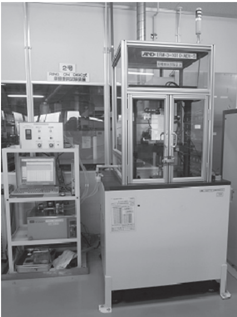
Photo 2. Ring-on-disk friction and wear test equipment
