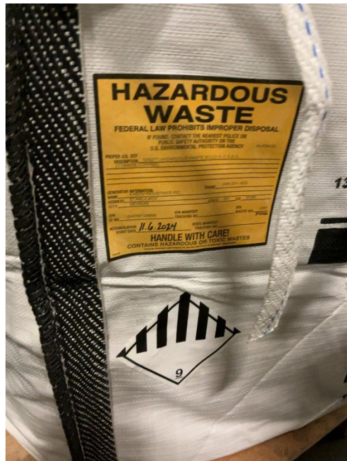
Photograph 8 Hazardous Waste labeling on super sack in Section 5- Warehouse CAA.
