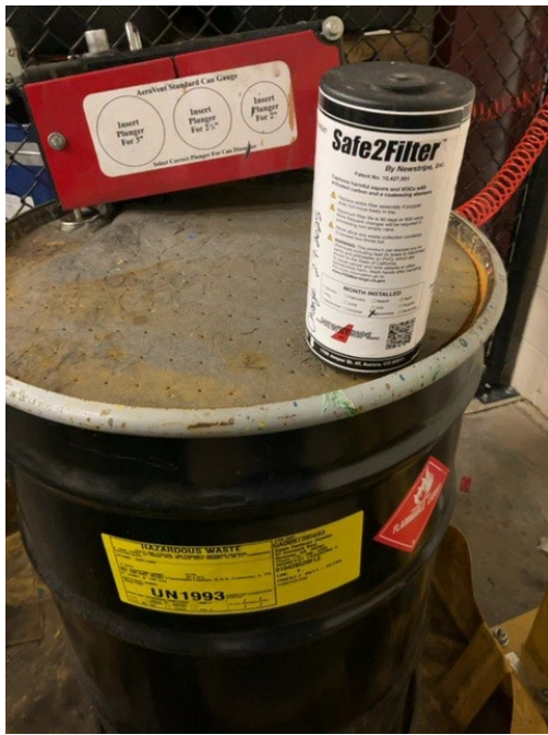
Photograph 13 Aerosol puncturing device in Section 5 Warehouse CAA.
