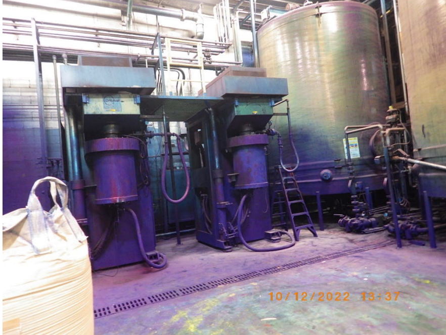
36: APOL0345 Description: Blue pigment media mills Location: Blue Room, south corner of Building 1 Camera Direction: North Date/Time: 10/12/22, 1:37 p.m.
