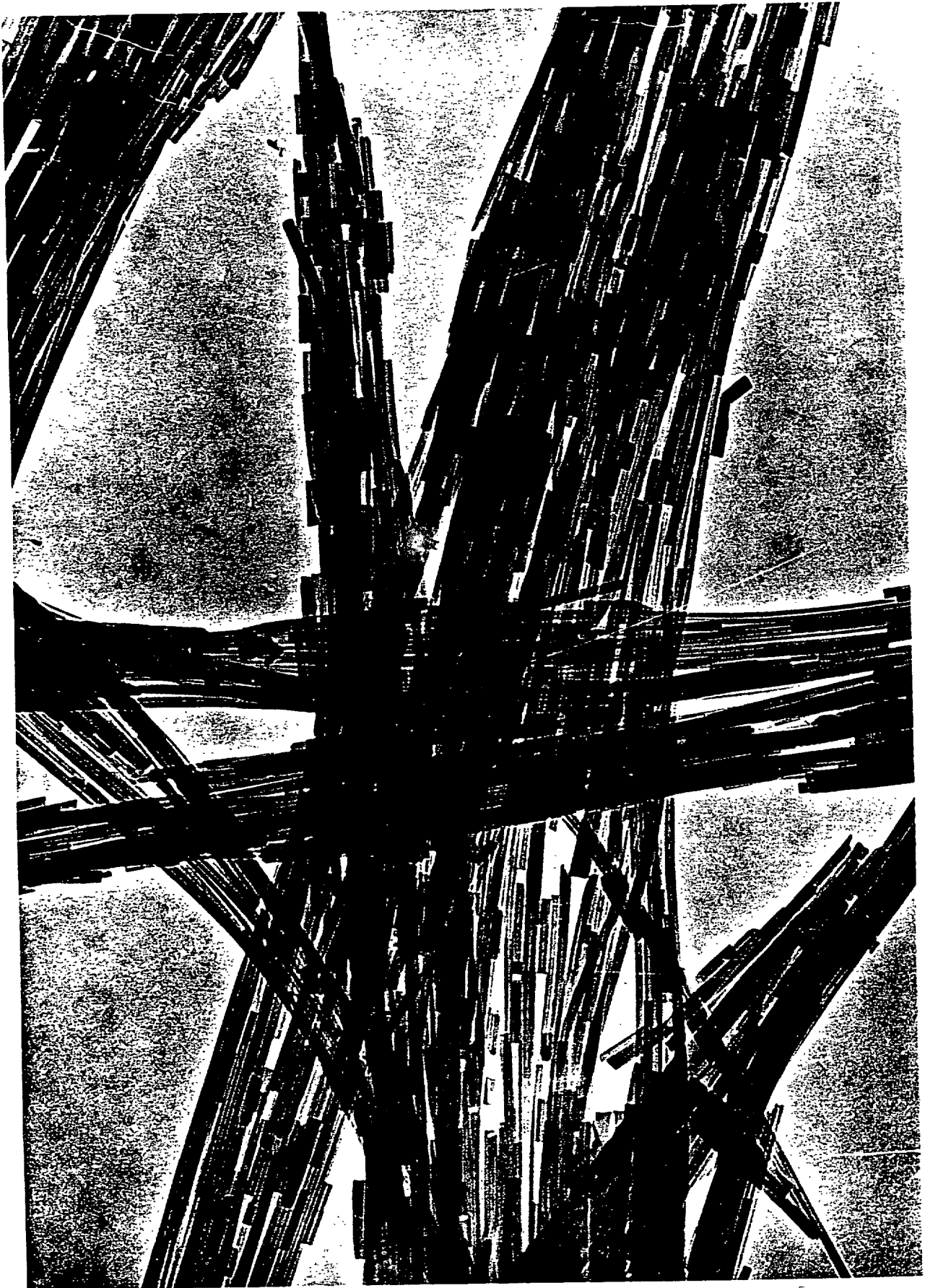
Fig. 6 - Electron Micrograph of dry processed asbestos fibers
