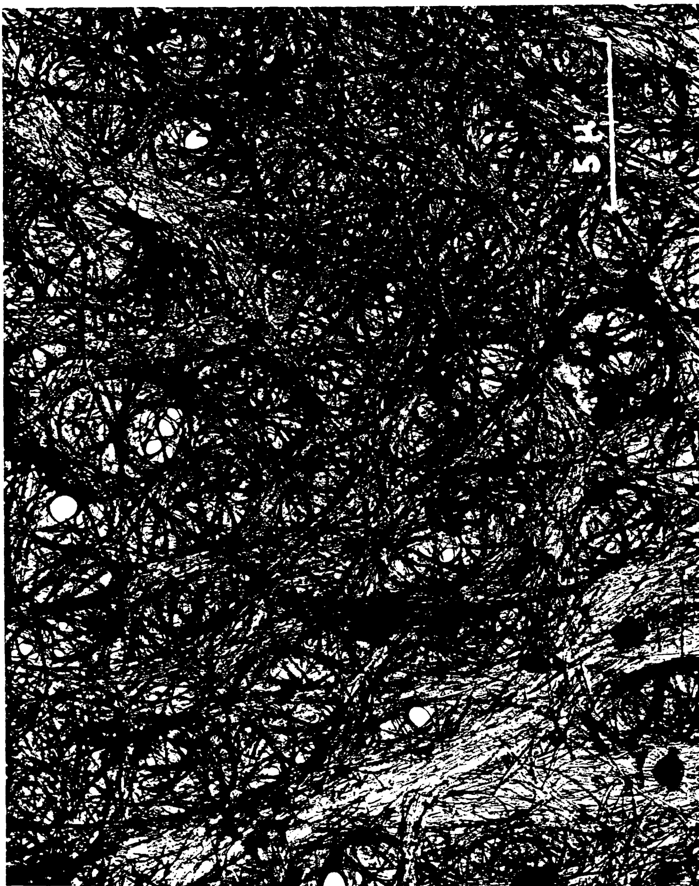
Fig. 5 - Electron Micrograph of typical Calidria asbestos fibers
