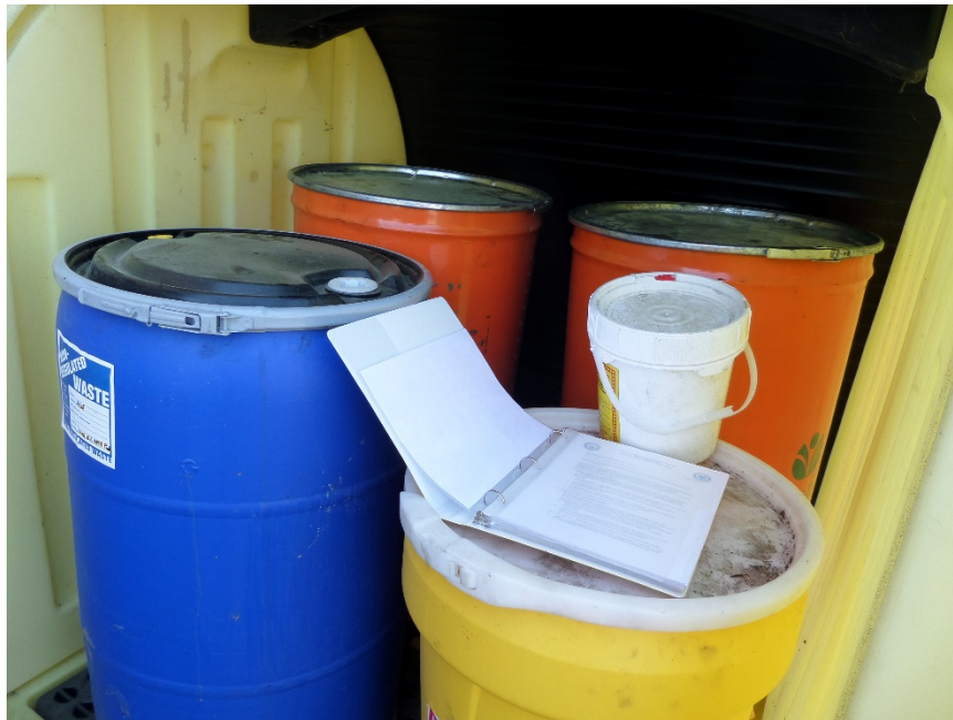
Photograph 11: Air Ground Equipment Maintenance Area - SAA 001 One 1-gallon empty container labeled hazardous waste-lead, one 30-gallon hazardous waste container of jet fuel contaminated absorbent pads, one 55-gallon container of used oil contaminated absorbent pads, one 55-gallon container of used oil drained filters and one 55-gallon container of diesel filters.
