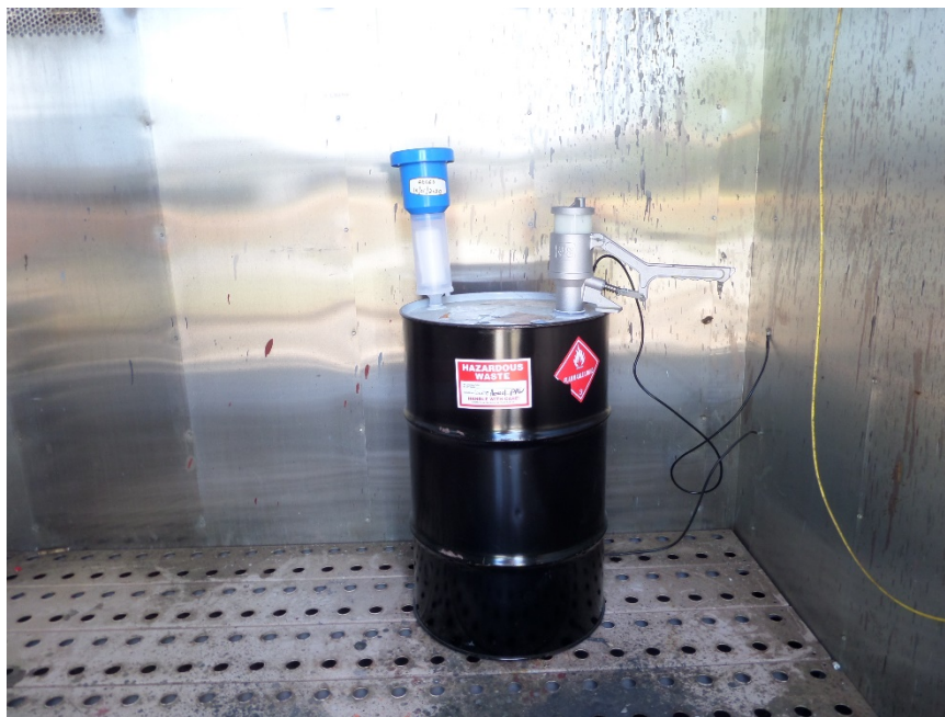
Photograph 6: Shelter B- Hazardous waste accumulation container with aerosol can puncturing device used to empty hazardous waste paint aerosol cans generated at the facility.
