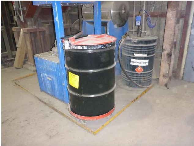
Photo 22: Finishing Dept. – Still bottoms container and solvent recovery unit
