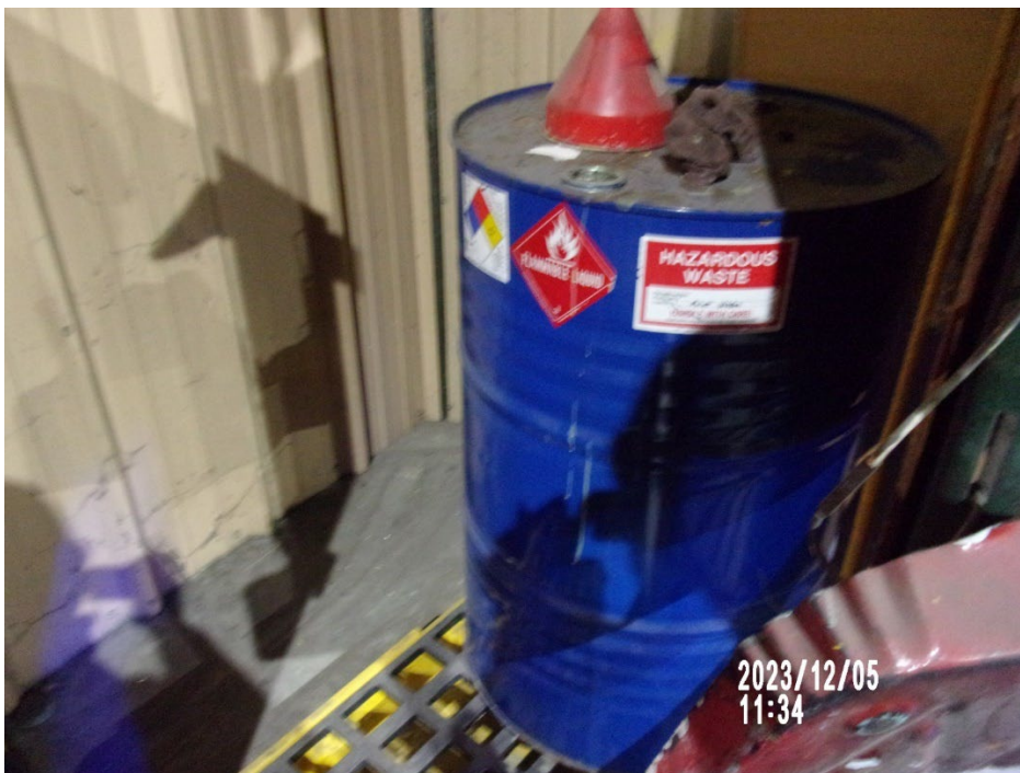
Photo 33: 55-Gallon Hazardous Waste SAA for Paint Waste.
