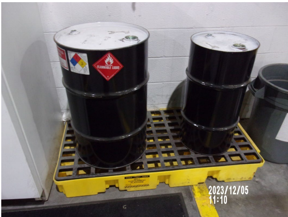
Photo 28: SAA Hazardous Waste Containers for the Facility Laboratory Containing Waste Styrene (55-Gallon Container) and Waste Methylene Chloride (30-Gallon Container).
