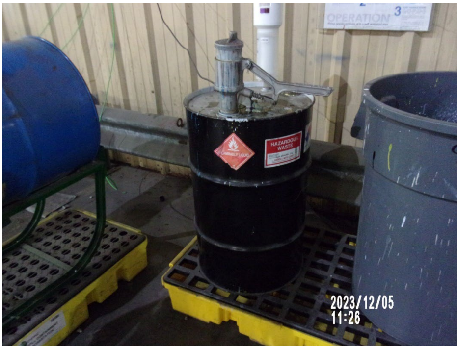
Photo 30: Aerosol Can Puncturing Device Affixed to Metal 30-Gallon SAA Container.
