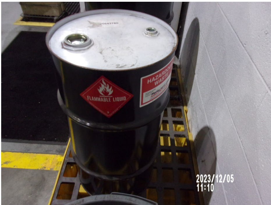
Photo 29: Labeling and Marking on the 30-Gallon Waste Methylene Chloride Container.
