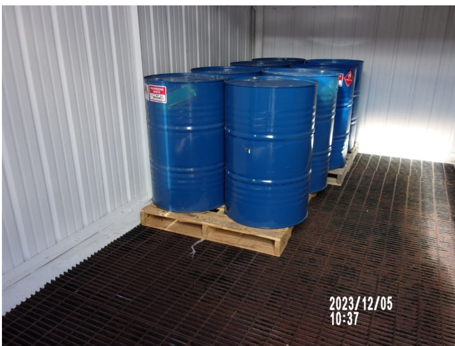
Photo 18: Third photo of the eight grouped metal 55-Gallon containers in the CAA. The inspectors were able to see the labels and markings but advised the facility to consider moving the containers away from the wall.
