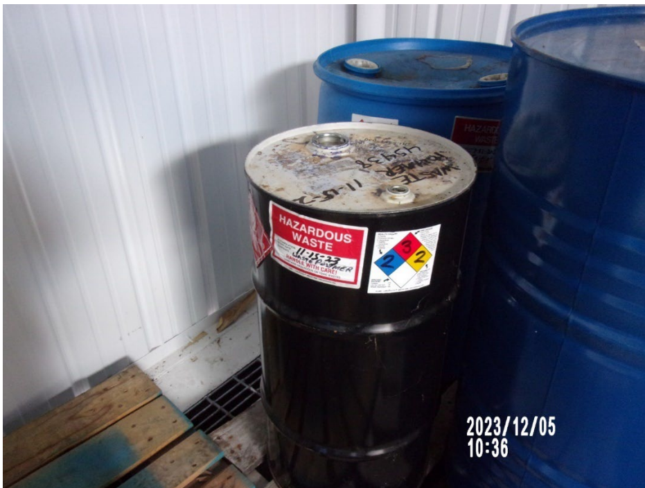
Photo 14: Metal 16-Gallon Hazardous Waste Container in the CAA. Plastic 30-Gallon Hazardous Waste Container is dated 7/31/2023 but has received an accumulation variance from KYDEP.
