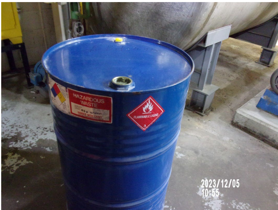
Photo 24: Metal 55-Gallon SAA Container in the Plant 1 Containing Waste Ethylbenzene and Water.
