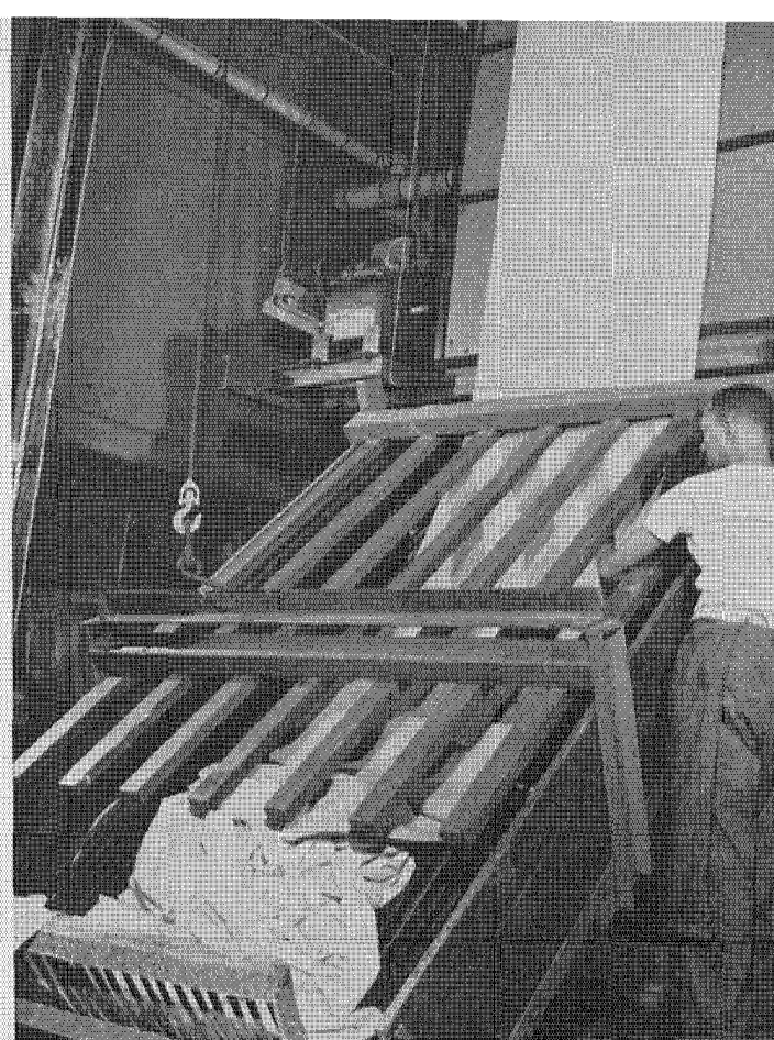
Treating cloth with durable Du Pont "Erifon" flame retardant. This excellent product was dropped because it was simply too expensive to apply to the fabric.
