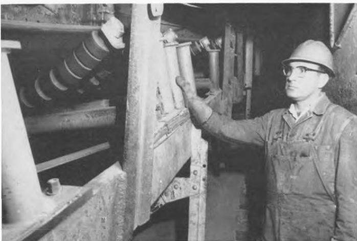
Kennecott's First Inventor-Suggester. Inventor Don G. Marsh, a machinist at the Nevada Mines Division, became the first employee to be granted a patent under the Employee Suggestion and Patent Plan. Mr. Marsh is shown here explaining how his impact-absorbing device reduces breakage of conveyor belt idler supports.
