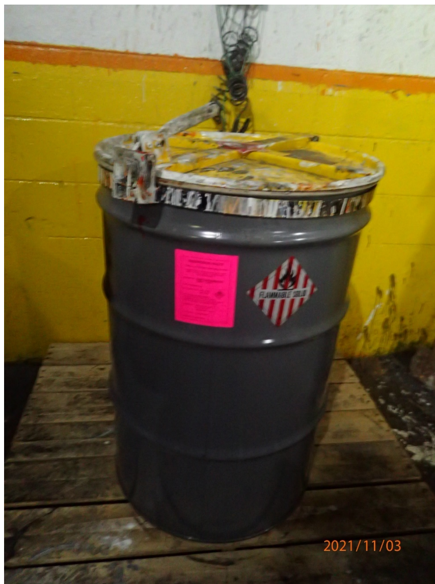
Photo 1: One (1) 55-gallon drum of paint contaminated debris in different, closed, labeled “Hazardous Waste”, and marked with an indication of hazard.
