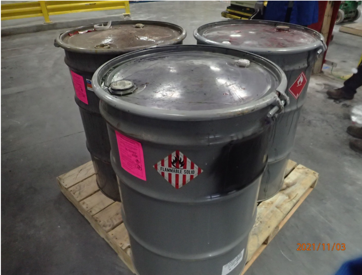
Photo 2: Three (3) 55-gallon drums of paint-contaminated debris generated from three different washes of machinery. The containers were closed, labeled, dated, and marked with an indication of hazard. The containers were on a pallet to be sent to the 90-day central accumulation area.
