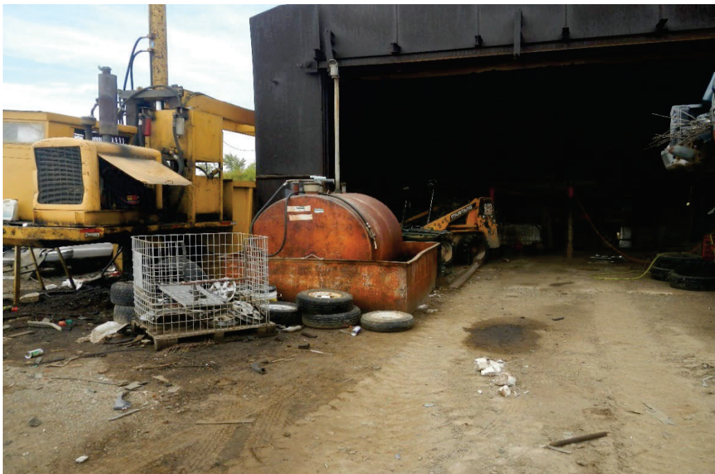
Photo 14, significant ground discoloration in the vicinity of the bale
