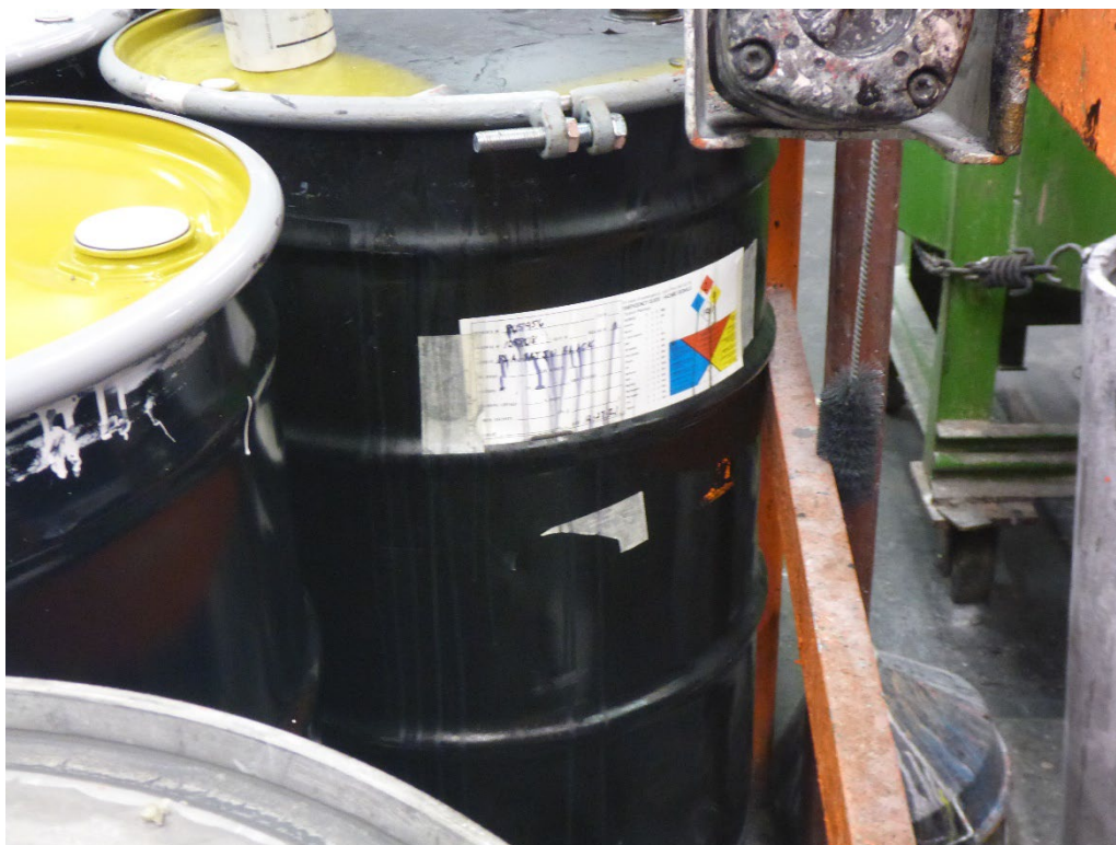
Photo 9: One of six 55-gallon drums of hazardous waste observed on portable secondary containment pallets in the Mix Room near the center of the room. The drum was not labeled as hazardous waste. The ink on the label had run, causing the values marked on the NFPA fire diamond to be illegible.
