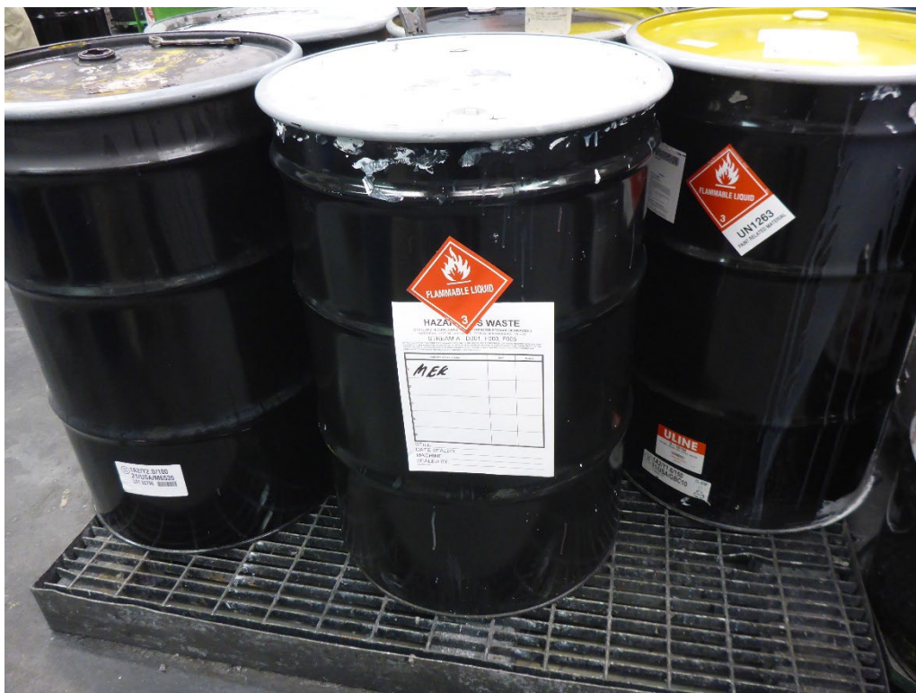
Photo 7: Three of six 55-gallon drums of hazardous waste observed on portable secondary containment pallets in the Mix Room near the center of the room. The drum on the left was not labeled as hazardous waste or marked with an indication of the hazards of its contents. The drum in the center was labeled as hazardous waste and marked with a flammable liquid DOT hazard placard. The drum on the right was not labeled as hazardous waste, but it was marked with a flammable liquid DOT hazard placard. None of the hazardous waste containers were marked to indicate their contents are toxic.
