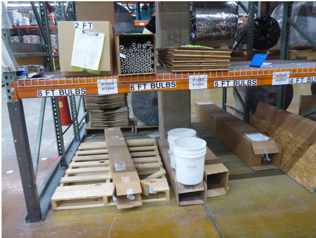
Photo 20: One box of 2-foot universal waste lamps, one box of 4-foot universal waste lamps, one box of 6-foot universal waste lamps and one box of 8-foot universal waste lamps in the Warehouse. All of the boxes were open. The boxes of 6-foot and 8-foot lamps were labeled as universal waste lamps, but no labels were affixed to the boxes of 2-foot and 4-foot lamps. Instead, these labels were located on a clipboard that had been placed on top of each container. The oldest universal waste label was dated 11/04/2021.
