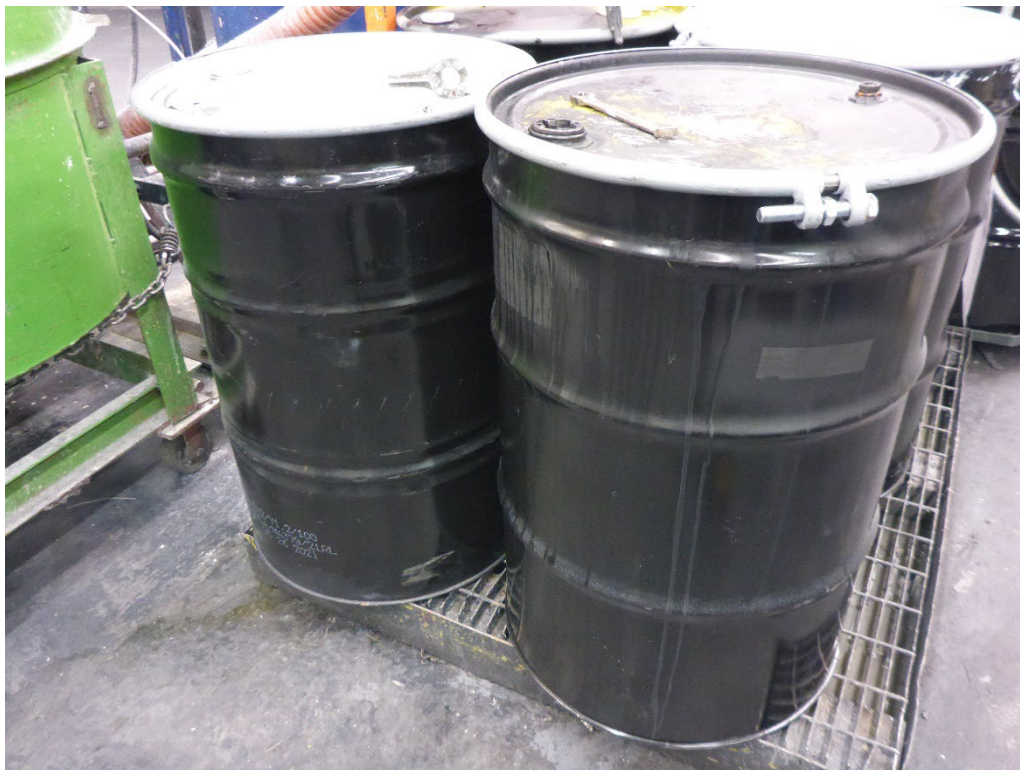
Photo 8: Two of six 55-gallon drums of hazardous waste observed on portable secondary containment pallets in the Mix Room near the center of the room. The drums were not labeled as hazardous waste, marked with an indication of the hazards of its contents, or marked with an accumulation start date.
