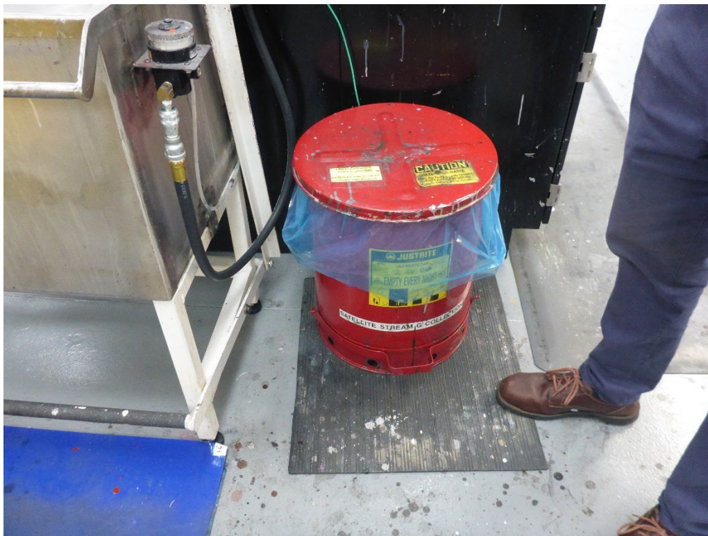
Photo 12: One of six 14-gallon step-to-open flammable cans in the Liquid Laboratory SAA for accumulating Stream G hazardous waste solids. The container is labeled “Stream G hazardous waste solids,” but it is not marked with an indication of the hazards of its contents. In addition, the original “oily rags” and “empty every night” labels are still visible on the container.
