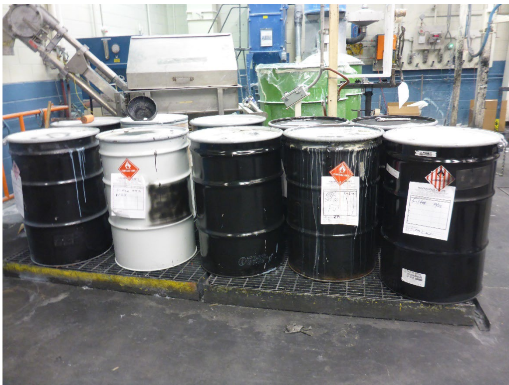
Photo 5: Ten 55-gallon drums of hazardous waste observed on portable secondary containment pallets in the Mix Room near the Distillation Unit. None of the containers were marked to indicate the contents are toxic.
