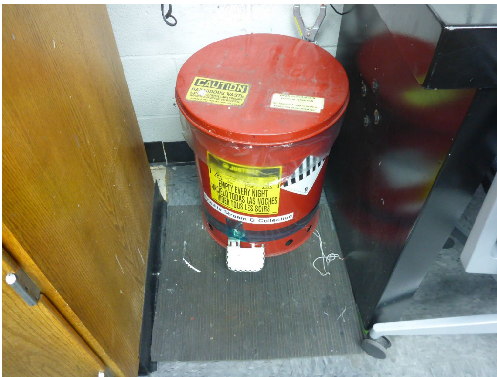
Photo 18: One 14-gallon step-to-open flammable can in the In-Process Laboratory SAA for accumulating Stream G hazardous waste solids. The container is labeled hazardous waste, but it is not marked with an indication of the hazards of its contents. In addition, the original “oily rags” and “empty every night” labels are still visible on the container.
