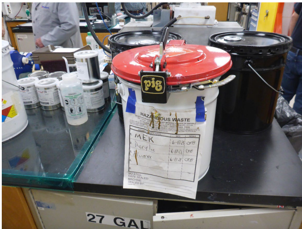
Photo 15: One 5-gallon container in the Color Laboratory SAA for accumulating Stream A High Water hazardous waste liquids. The container is labeled hazardous waste, and the hazards of the contents of the container are indicated using an NFPA fire diamond.
