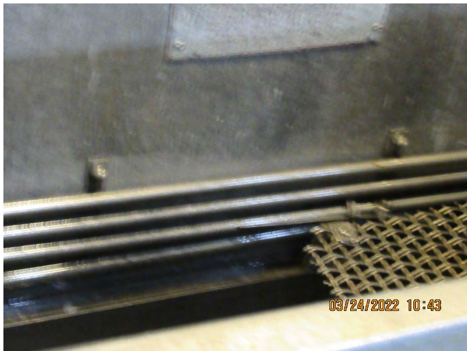
Photograph #8 – Vapor degreaser cooling coils capturing & returning solvent
