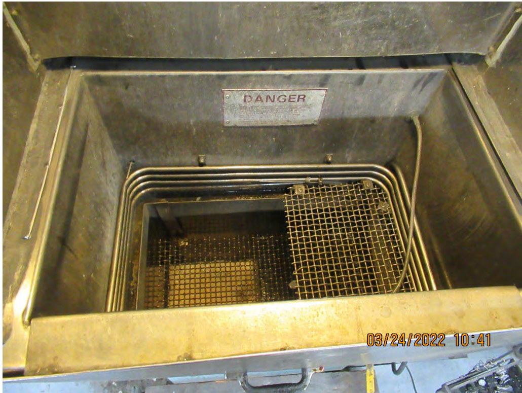
Photograph #8 – Vapor degreaser cooling coils capturing & returning solvent
