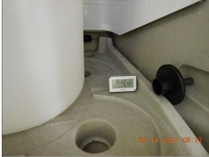
9: DSCN0968.JPG Location: Tilden and Empire Mine Photographer: Jonathan Moody Date/Time: 9/14/2022 8:22 AM Description: Non-NIST traceable thermometer at the location shown in photo 8.
