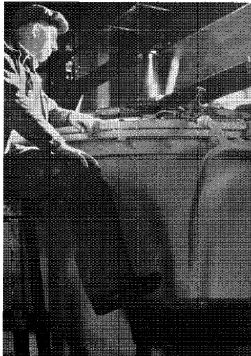
Nitration is a key process in many du Pont plants. Here, the operator is making nitroglycerine, a dynamite ingredient. Through a glass window he watches and controls with extreme care the reaction between glycerine and mixed nitric and sulphuric acids
