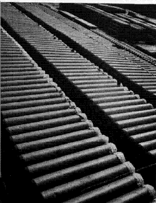
One important use for ammonia is in nitric acid manufacture, but it has many applications of its own. Compressed in the cylinders pictured here, it is shipped all over the world, to be used for refrigeration and other purposes.
