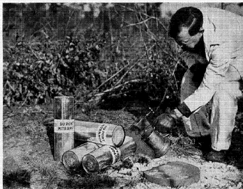
Even the flames from a blow-torch cannot explode this new blasting agent "Nitramon," as was demonstrated at Millville, N. J., to representatives of the press.
