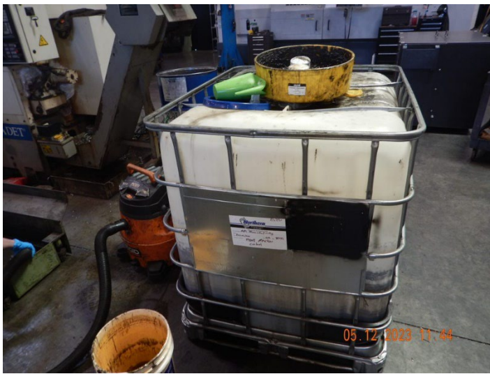
Photo #: 01 (DSCN0603) Description: Approximately 275-gallon intermediate bulk container holding used oil.
