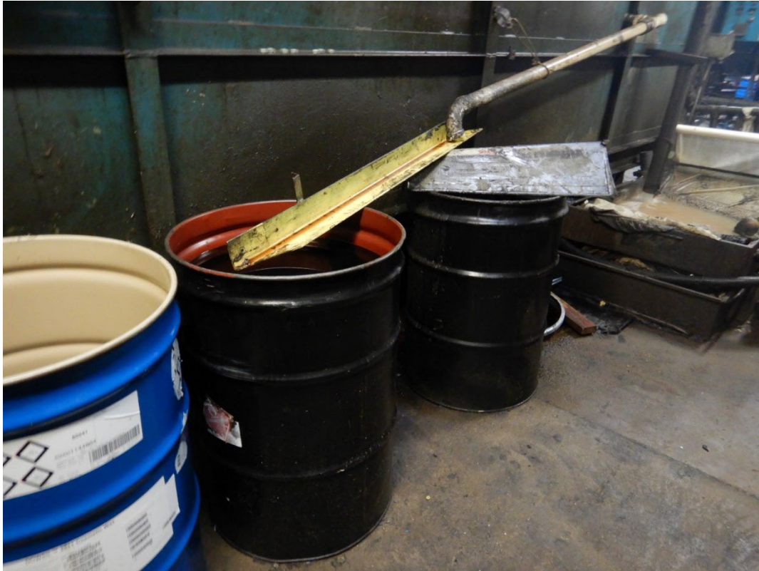
Rotary screen waste satellite accumulation area, adjacent to the wastewater treatment equipment. The two black drums contain rotary screen waste. Neither of the drums are labeled or closed.
