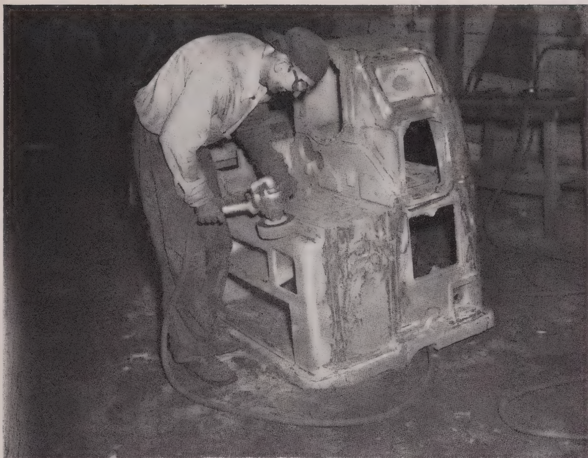
Figure 6.—Removing rough spots from casting by portable grinding.
