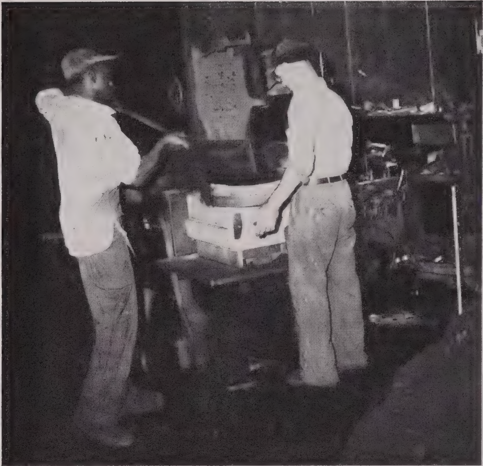
Figure 2.—Machine molding of small castings. Molder's helper at the left is shoveling sand into a screening device to provide facing sand for the mold. Pile of heap sand is in the right foreground.
