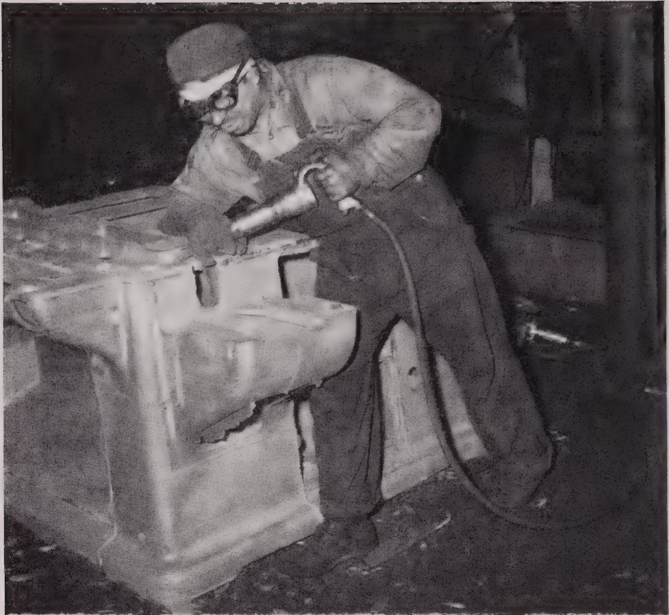
Figure 8.—Removing excess metal from casting by pneumatic chipping.
