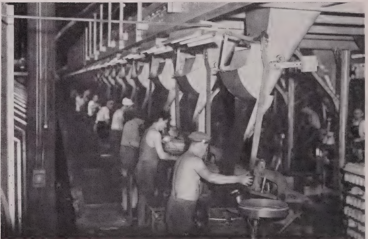
Figure 3.—Line of machine molders. Molding sand is provided by an overhead conveyor system. Finished molds are taken to a central pouring area by the conveyor directly behind the molders.
