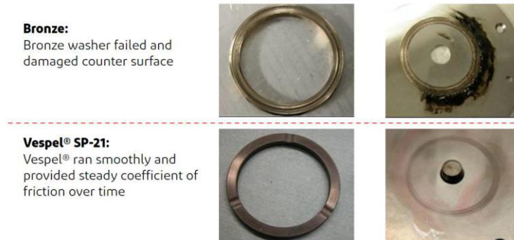
Figure 23: Vespel® thrust washer in comparison to bronze
