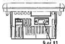
RS-232 (DH-485 or DF1) without additional RS-232 Port
