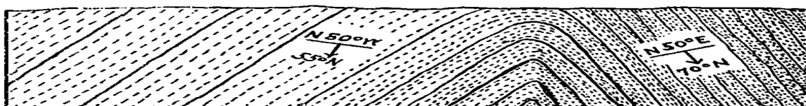
Figure 13 Section in railroad cut not far east of Talcville, across the nose of a pitching isoclinal fold in hard gneisses.
