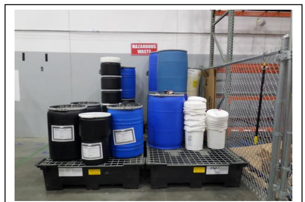
Cardinal Health. 90-Day Area. Hazardous waste area. Containers closed, labeled, and dated. Photograph 4 taken at 12:06 p.m.
