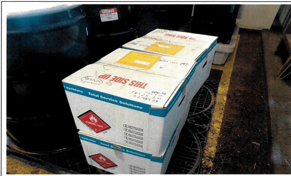
Naval Air Station Whiting Field. Main 90-Day or Less Accumulation Area Building 3156. Observed four boxes stacked two high on a poly pallet. Inspectors could not observe the hazardous waste label on each of the bottom boxes due to the double stacking. The facility removed the two top boxes revealing the labels. Photograph 1 taken at 10:16 a.m. WK.
