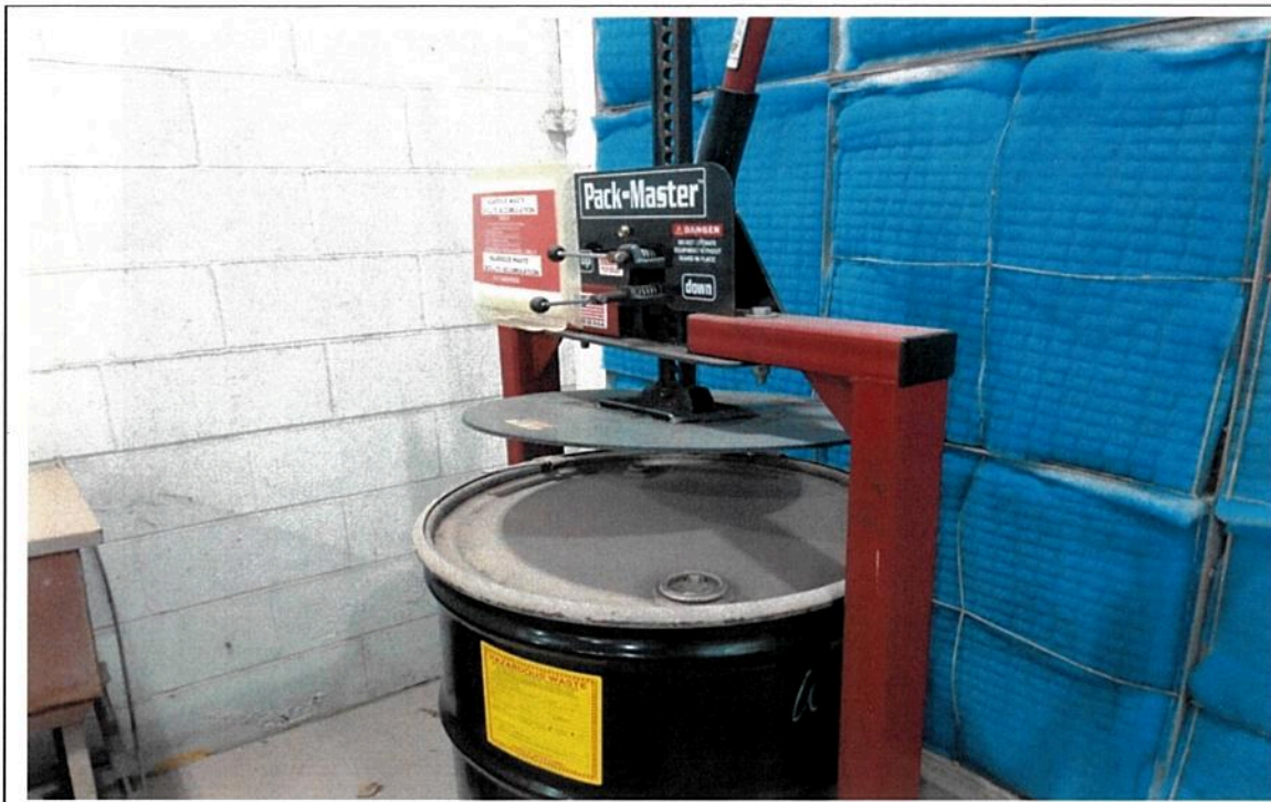
Naval Air Station Whiting Field. Paint Booth and Corrosion Building 3024. Observed one 55-gallon container under a manual drum compactor. Container was on a pallet. Photograph 3 taken at 11:16 a.m. WK.
