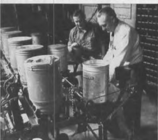
A & M's newly developed grass seeder can be used for reseeding abandoned cropland and renovating depleted rangelands. R. D. Barmington (right) is acting head of Mechanical Engineering.
