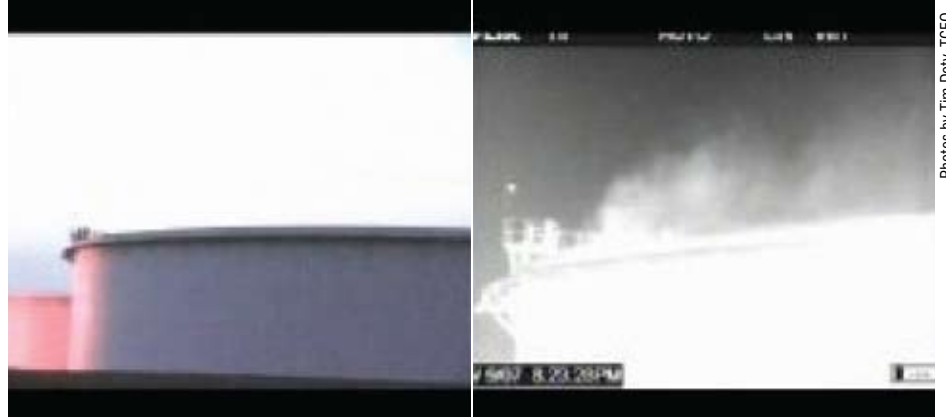
To the naked eye, nothing appears amiss at this tank facility in Nederland. But the lens of an infrared imaging camera (right) tell a different story—hydrocarbons escaping into the atmosphere of East Texas. This new camera technology is helping to advance mobile monitoring.
