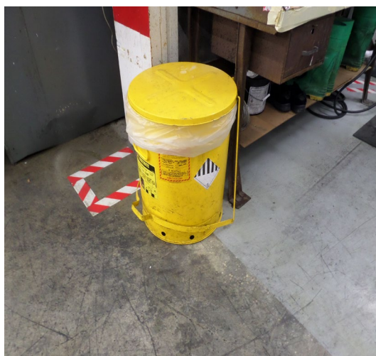
H & S. Chem Film/Chromate Room. Observed the 30-gallon step can had a Class 9 DOT label. Photograph 2 taken at 10:20 a.m.
