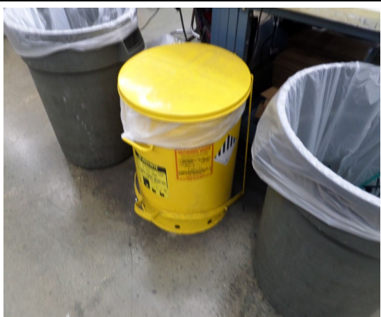
H & S. Paint Department. Observed the 30-gallon step can had a Class 9 DOT label. Photograph 3 taken at 10:20 a.m.
