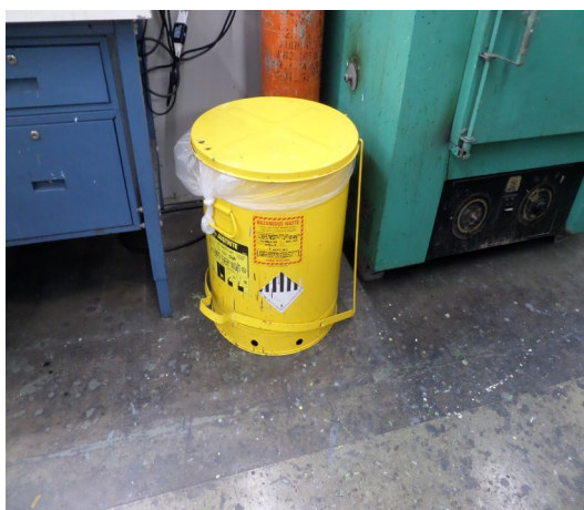
H & S. Paint Department. Observed the 30-gallon step can had a Class 9 DOT label. Photograph 4 taken at 10:22 a.m.
