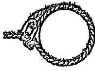
Bad—Left on running line can work loose
