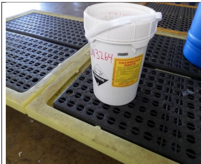
CCSFS. Permitted Storage Building 44200, Acidic Waste Bay. The inspectors observed a five-gallon container of hazardous waste (D002, D007) not marked or labeled with a toxic hazard indicator. Facility marked the word toxic on the container. Photograph 3 taken at 10:24 a.m.
