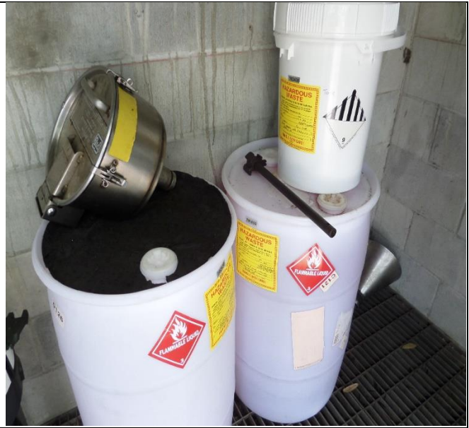
CCSFS. Chemistry Laboratory, Petroleum Solvent/Oxidizer CAA. The inspectors observed two 30-gallon containers and one five-gallon container of hazardous waste not marked or labeled with a toxic hazard indicator. Facility marked the word toxic on the container. Photograph 10 taken at 2:02 p.m.
