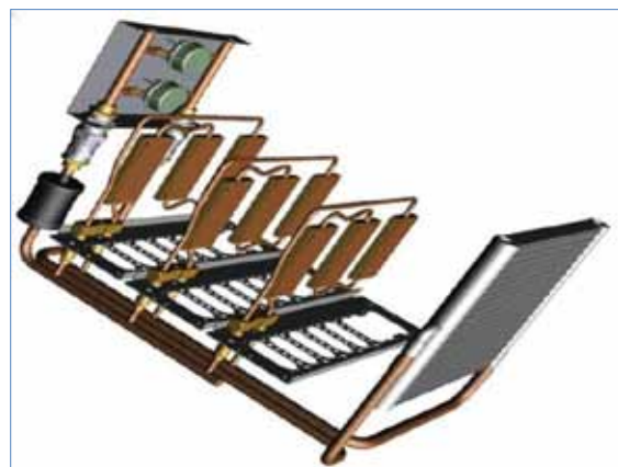
Figure 8. Modular VDF cooling system for hybrid vehicle powertrain inverter
