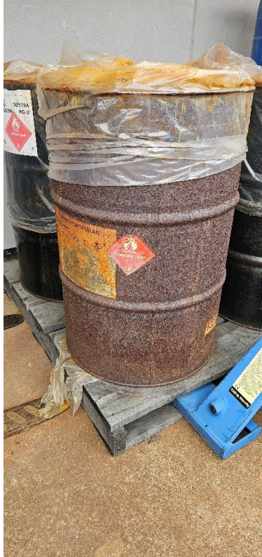
Figure 11: In the back pad area, one 55-gallon drum of Tetrahydrofuran was observed to be extremely corroded and potentially unusable in the condition observed.
