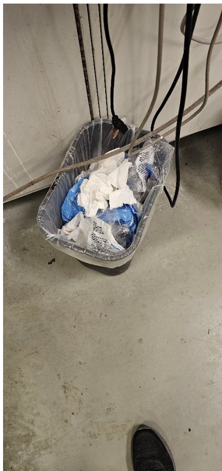
Figure 4: Hazardous waste lab PPE, hazardous waste lab equipment, and hazardous waste chemical-stained rags observed stored in municipal waste garbage can.
