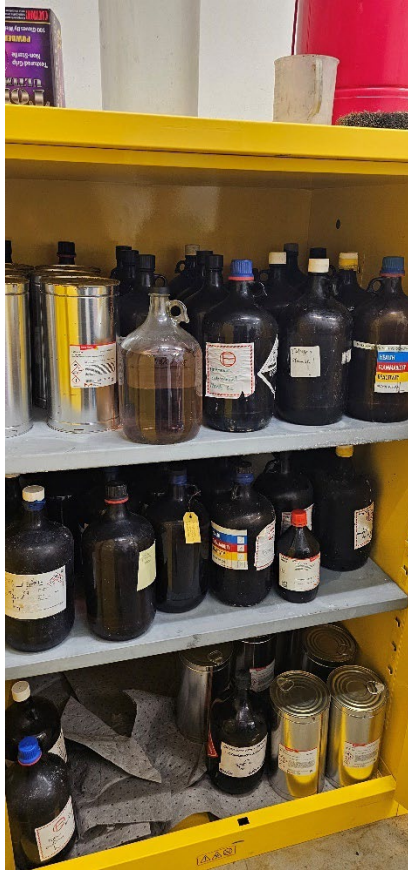
Figure 8: In the mixing room flammables cabinet 1, one container labeled as “unknown substance - needs GC,” the container was unidentified at the time of the inspection and a hazardous waste determination was not done. The container had a corrosives placard on it and was incompatibly stored with ignitable materials.
