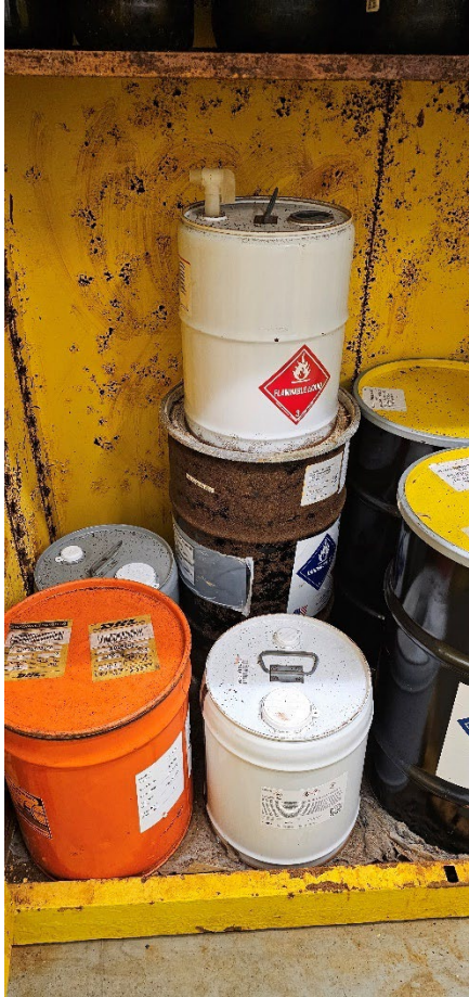
Figure 9: In the mixing room flammables cabinet 2, one 35-gallon drum of magnesium powder was observed to be severely degraded and had flammable liquid stored on top of the drum. The magnesium powder was labeled “dangerous when wet” and “spontaneously combustible.”
