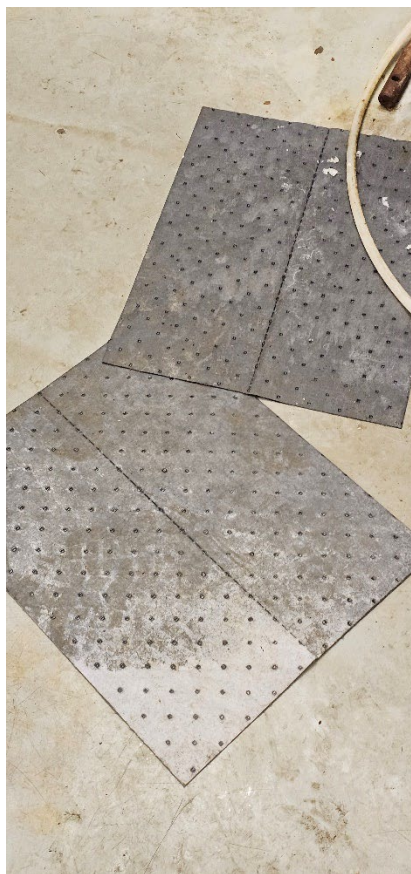
Figure 7: Absorbant pads observed in the polyramics lab were severely stained and saturated and no longer sufficient to properly contain hazardous waste spills.
