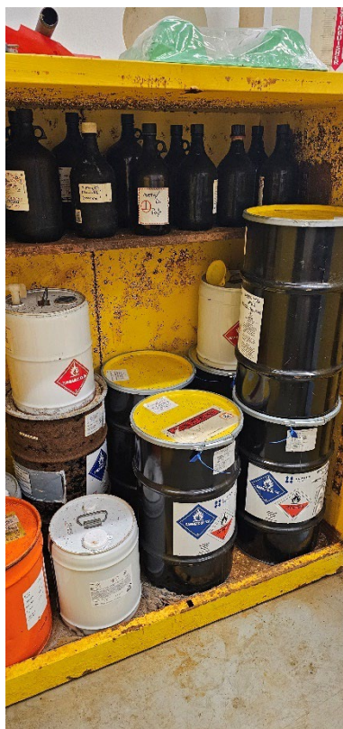
Figure 10: In the mixing room flammables cabinet 2, many of the stored chemical containers showed signs of corrosion and degradation. The corroded magnesium powder drum can also be seen in the figure.
