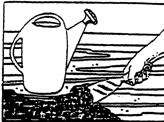
Sketch I. After wetting felt, an stiff-bladed scraper is used.
