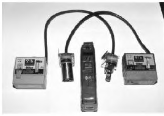
Figure 1. Pictorial view of Cowl sampler (left), BGI sampler (right) and Real-Time Dust Monitor (centre)
