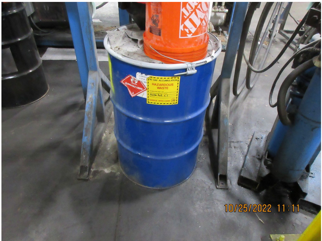
Photo 1 – Drum of Hazardous Waste “Huckle Pack Oil” in South Extrusion Area SAA
