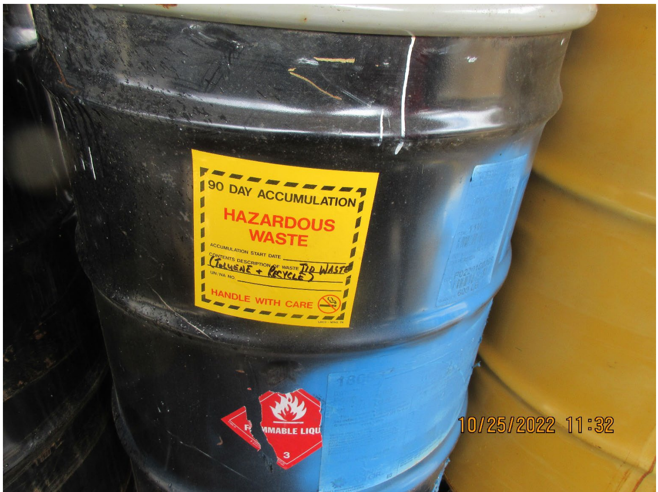
Photo 5 – Missing Accumulation Start Date on Drum in CAA
