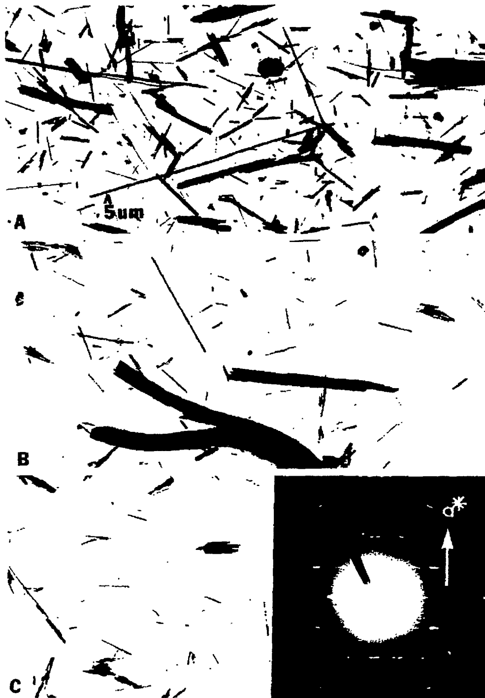
FIG. 1. Montage of transmission electron micrographs of UICC Rhodesian fiber (A), RG 144 Calidria fiber, as received (B), and RG 144 milled for 1200 sec (C). Fiber in A is about 5 \mu\text{m} in length. Magnification for each micrograph is the same. The Rhodesian fiber specimen consists of many fibers greater than 5 \mu\text{m} in length; RG 144, as received, contains fewer long fibers, as does the 1200-sec milled preparation. The selected area electron diffraction pattern (inset in C) shows the chrysotile structure was retained even after the 1200-sec milling treatment.
