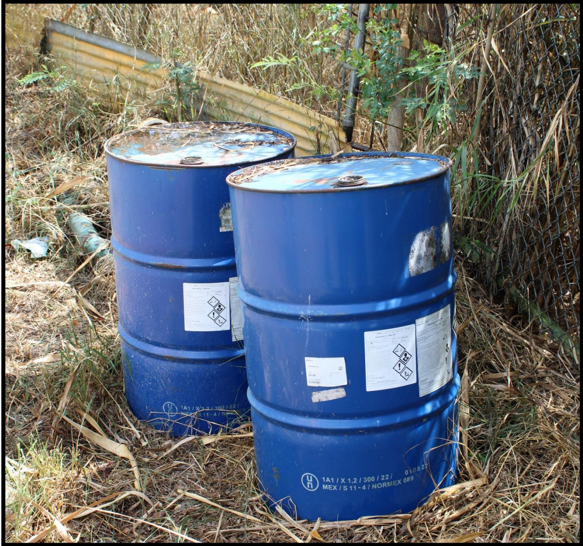
Picture 10 shows two 55-gallon metal drums exposed to rain and lacking secondary spill containment.
