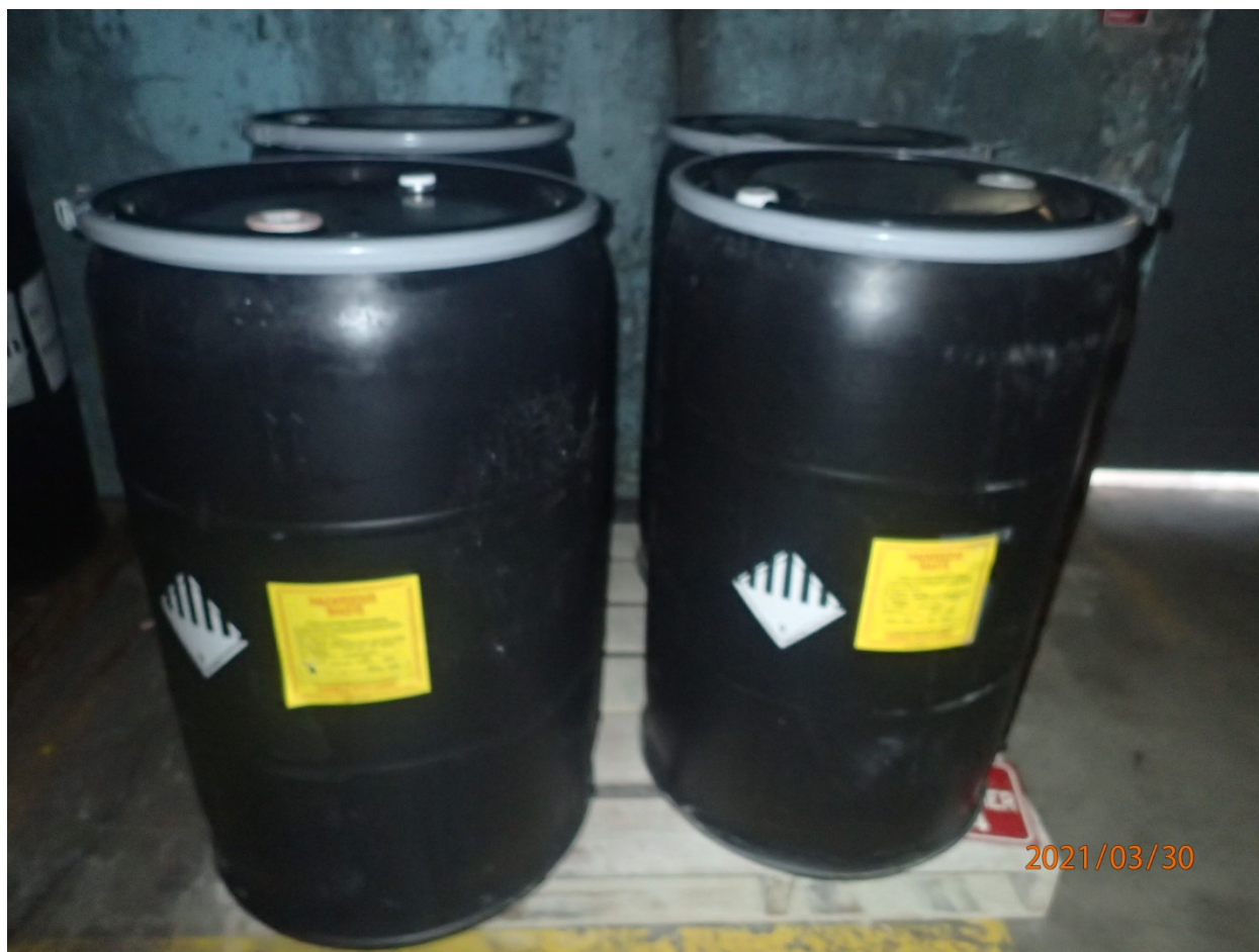
Photo 8: Pen 1 in Magnolia Plant. 55-gallon drums of Hazardous Waste Paint - Waste Blasting Media - D008.
