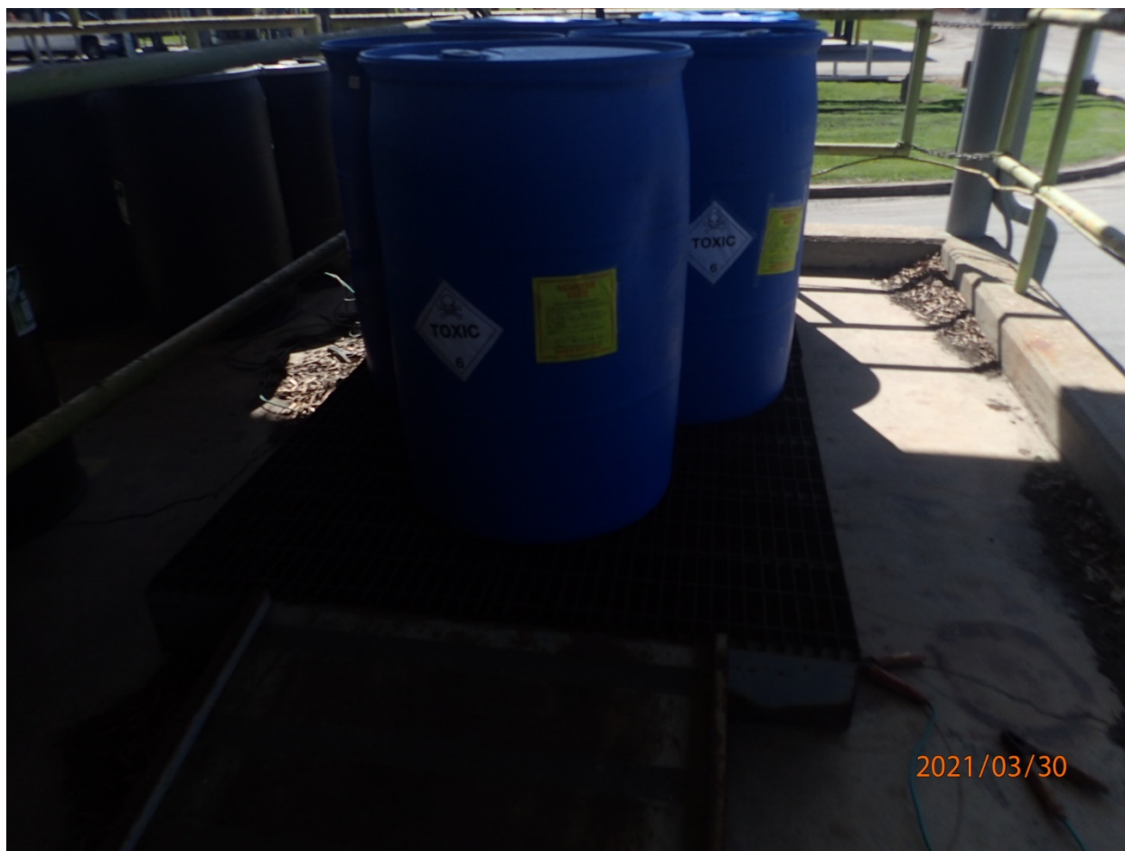
Photo 15: 55-Gal drums of Hazardous Waste Toxic FR Mix - D004, D007. Designated CAA in Dock Area. Magnolia Plant.
