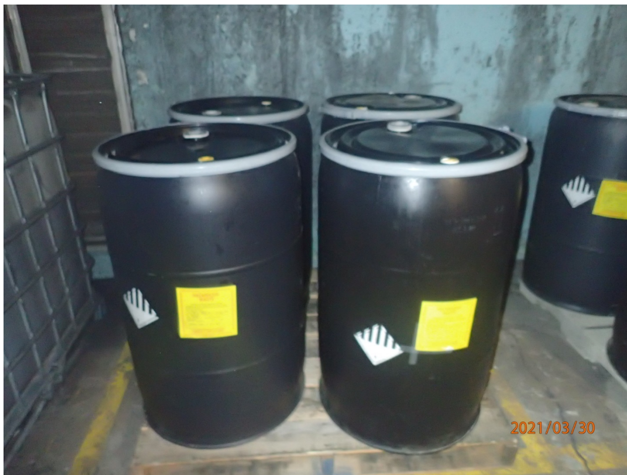
Photo 5: Pen 1 in Magnolia Plant. 55-gallon drums of Hazardous Waste Paint - Waste Blasting Media - D008.
