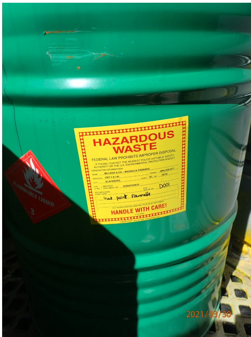
Photo 22: Close up of hazardous waste label of 55-gal drum labeled D001 Hazardous Waste Used Paint. Magnolia Plant.
