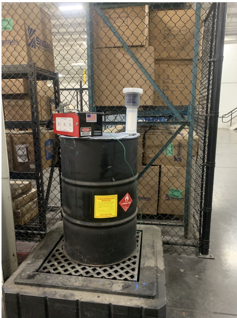
Photo 24: Photo taken by Rob Wallace, Environmental Manager at Allen Plant. 55-gal drum of Hazardous Waste – Paint with aerosol can puncture device.
