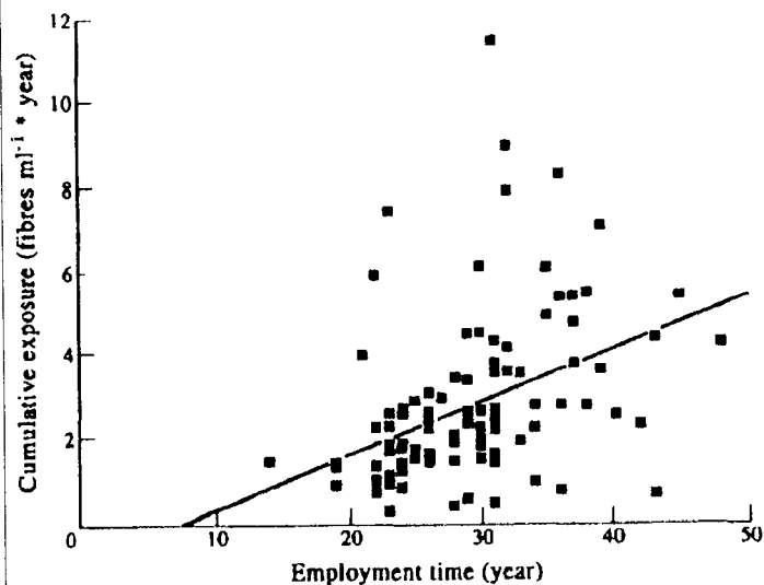
Fig. 4. Correlation employment time vs cumulative asbestos exposure for 103 vehicle mechanics: y = -0.793 + 0.123x ; r = 0.41 .
