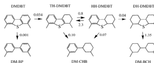
Figure 3. Mechanism of 4,6 Dimethyl Dibenzothiophene HDS and Relative Reaction Rates.
