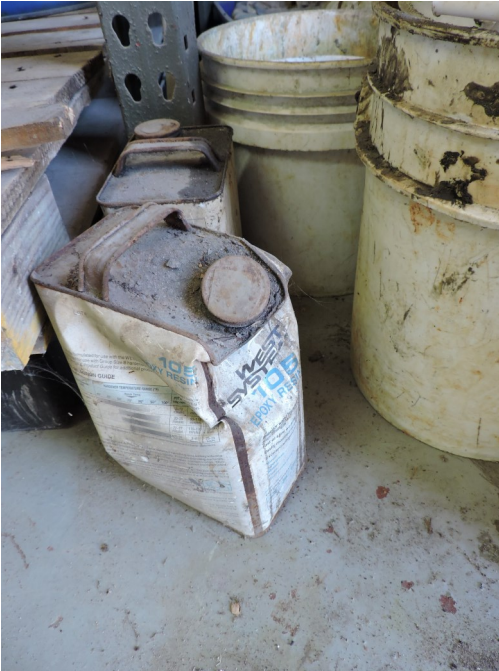
Picture 11 — Epoxy subarea—Here, two (2) containers with epoxy resin were observed. At the time of the inspection, one of them was observed in bad condition, corroded and with dust.
