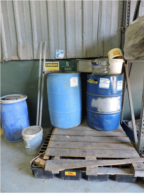
Picture 9 — Used oil subarea—Here, the 55-gallon plastic container was empty, while the 55-gallon blue steel container was observed labeled as used oil, and was labeled as non-regulated waste, as well.
