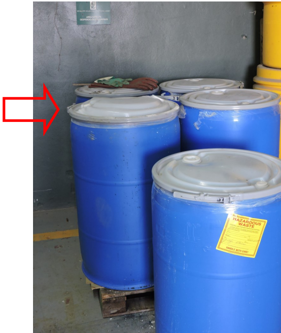
Picture 5 — SAA HW-2 subarea— Here, five (5) 55-gallon blue plastic containers were observed. Just one of them was labeled as hazardous waste, nevertheless, a pictographic label nor indication of the hazard was not observed. One of them was observed swollen.
