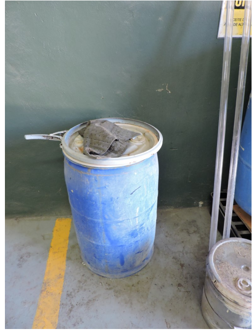
Picture 10— Silver sludge subarea— This container was not labeled, a pictographic label nor indication of the hazard was not available, and the date was not available, as well. Nevertheless, it was informed by the facility representatives that the latter contains silver sludge.
