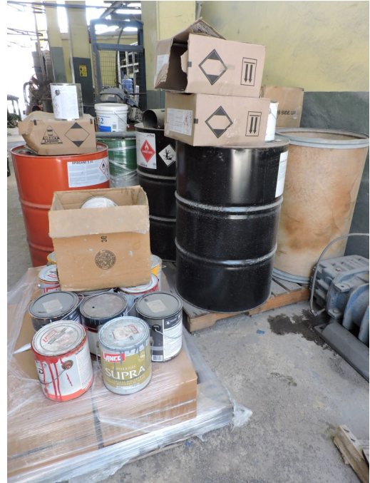
Picture 12 — In-front of flammable (cage-like) Area—While walking from the 90-day HWAA to the WWTP Area, I observed an area with concrete floor and ceiling with approximately thirteen (13) 1-gallon paint containers. These containers were observed corroded and with dust.
