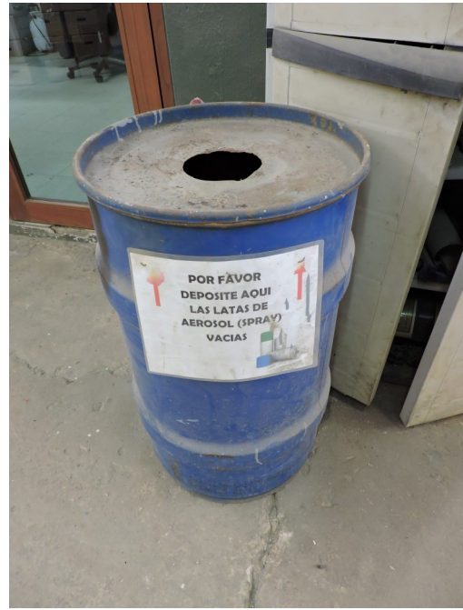
Picture 2 — Mechanical Shop Subarea— Here, a 30-gallon container was observed. The latter was labeled as Empty Aerosol cans and was observed open, with regular waste mixed with aerosol cans.
