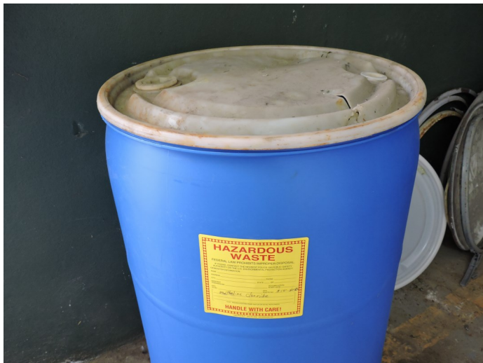
Picture 5 — SAA HW-2 subarea— Here, five (5) 55-gallon blue plastic containers were observed. Just one of them was labeled as hazardous waste, nevertheless, a pictographic label nor indication of the hazard was not observed. One of them was observed swollen.
