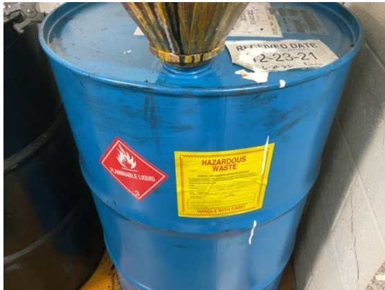
Photo 1: 55-gal container of waste ink. Container was closed, labeled “Hazardous Waste”, and marked with an indication of the hazards of the content.
