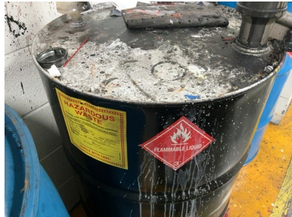
Photo 2: 55-gal container of aerosol can liquid with puncture device on top. Container was closed, labeled “Hazardous Waste”, and marked with an indication of the hazards of the content.
