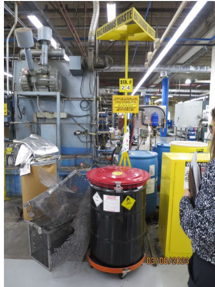
Photo #2 – Building 2- 55-gallon container of hazardous waste chromium salt and debris.
