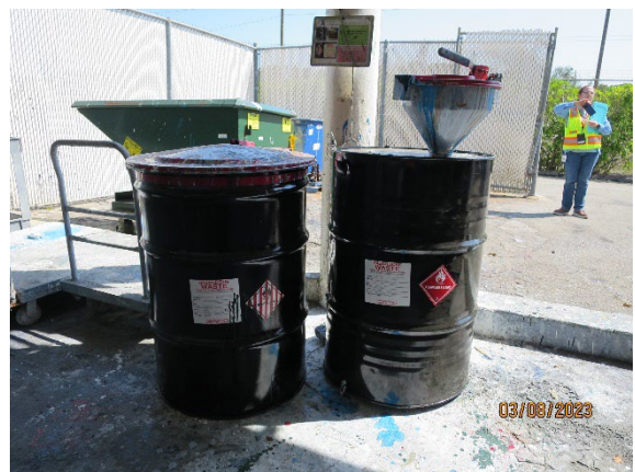
Photo #8 – Building 9 – two 55-gallon SAA hazardous waste containers located outside the building.
