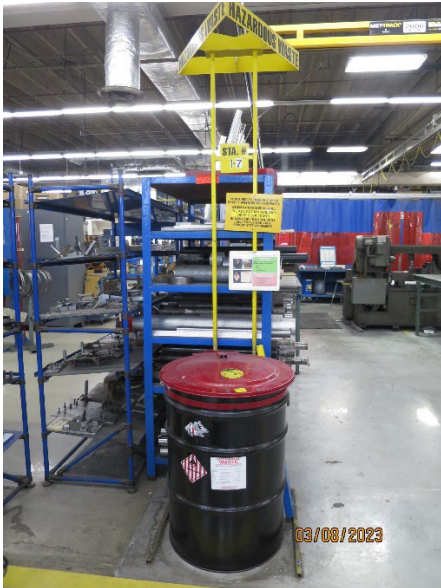
Photo #1 – Building 1- a 55-gallon container of waste acetone and filters, flammable solids.
