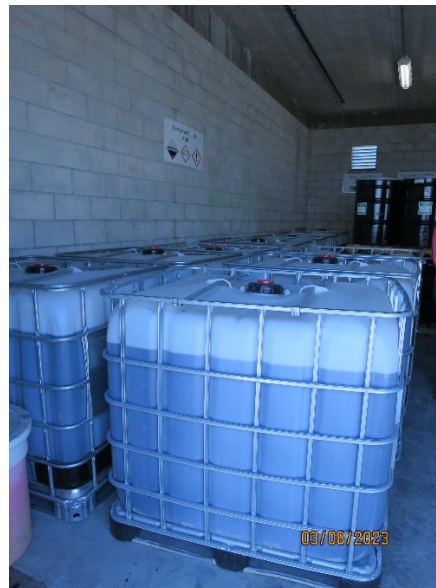
Photo #4 – CAA Building – 250-liter totes of corrosive waste marked and dated.
