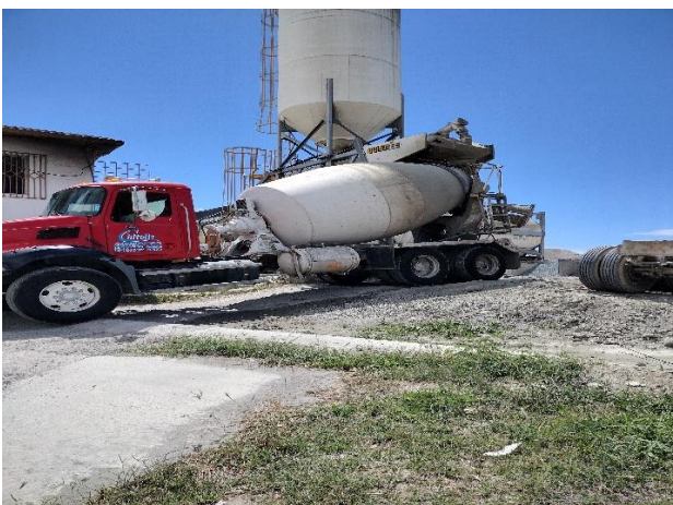
IMG 6311 -Truck in product bay being loaded with Ready-mixed concrete to be delivered to client construction site in the field.
