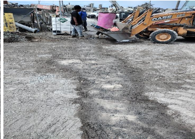
IMG 6838 -Dry-weather flow from area of RMCP towards central area of Facility carrying pollutants.
