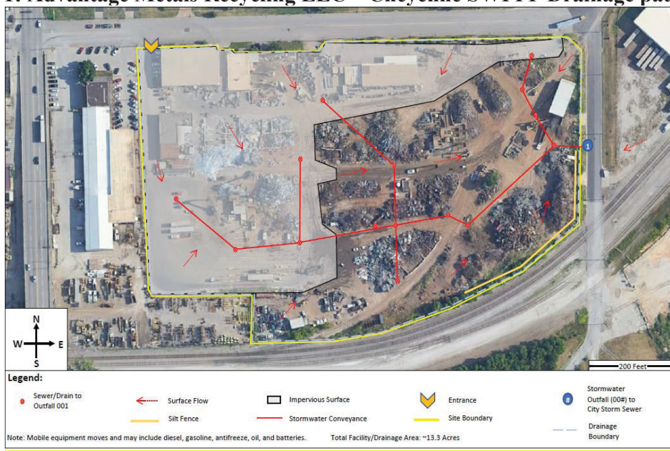
Figure 1: Advantage Metals Recycling LLC – Cheyenne SWPPP Drainage patterns map.
