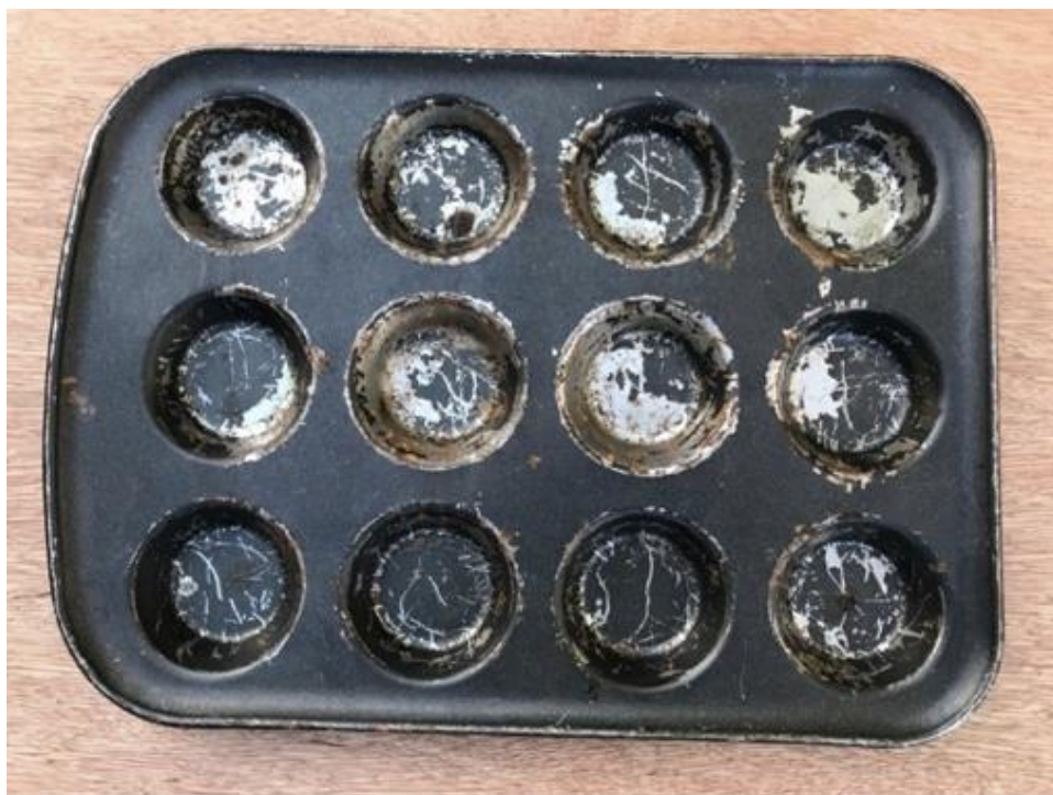
Figure E.5. Bun tin with severely degraded coating during prolonged use.
