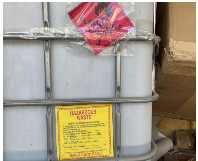
Picture 20 - GOV. JUAN F LUIS HOSPITAL, ST. CROIX— At the Hospital Backyard Area, the one (1) 330-gallon tote containing “Discarded Hand Sanitizer” was also identified with its hazard communication pictogram as, “Flammable Liquids,” and dated with its accumulation start date of May 30, 2023.
