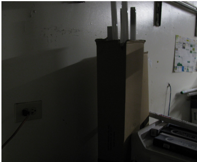
Picture 7 - GOV. JUAN F LUIS HOSPITAL, ST. CROIX- At the Universal Waste Storage Area, there was one (1) cardboard box with twenty-one (21) 4-foot spent fluorescent lamps, open, not labeled as “Universal Waste,” or dated , and no means to that prevents breakage and releases of hazardous constituents.
