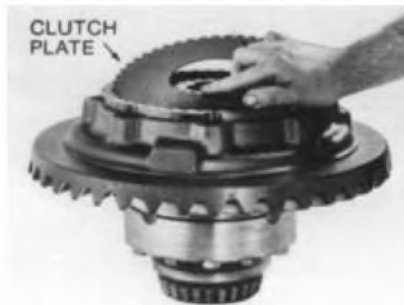
Installing External-Splined Friction Plate
