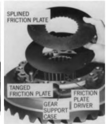
Removing Tanged and Splined Friction Plates
