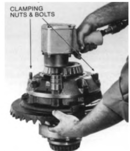
Removing Case Cover (with clamping nuts and bolts installed)
