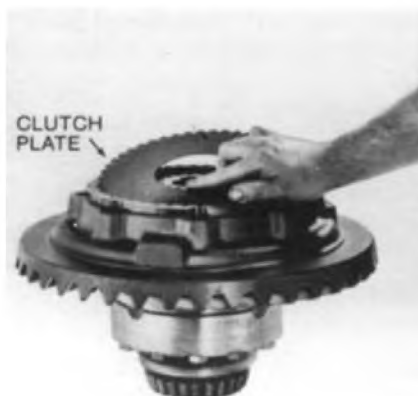
Installing Clutch Plates Individually (Permanent CTD Only)
