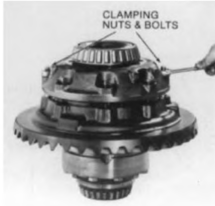
Removing Clamping Nuts and Bolts
