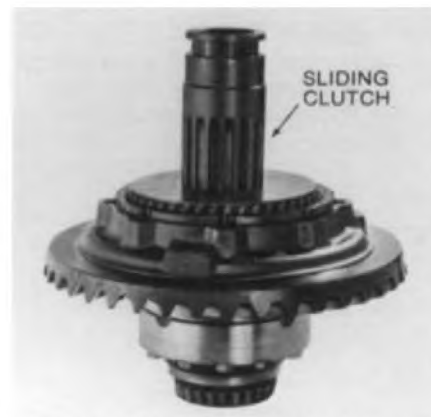
Aligning internal-Splined Friction Plate with Sliding Clutch
