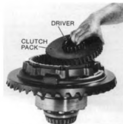
installing Clutch Pack and Driver Assembly (Permanent CTD Only)
