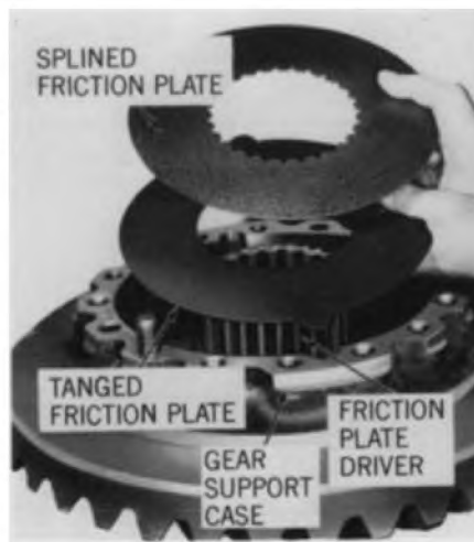
Installing Friction Plates
